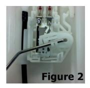
This fuel module ships with the arm detached from the module. To assemble float arm onto the fuel module insert the float arm into the hole (see Figure 1) and rotate the arm down so it engages the 2 clips on the bracket (see Figure 2). Ensure that it has a full range of motion and the float arm does not contact the body of the fuel module.
