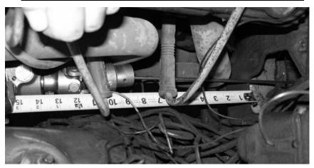
2) Transfer above measurement onto steering column.
