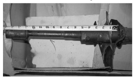
3) Add 1.5" to the measurement to allow for steering coupler engagement. This is where you will cut the steering column. *It is a good idea to leave the column 1" long to test fit, then cut to final length for installation.*
