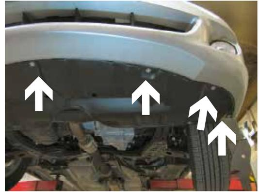
2. Using the 10MM socket remove seven metric bolts on the bottom edge of fascia.
