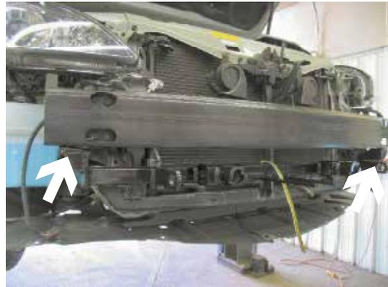
10. Reinstall molded styrofoam on the front of metal bumper and fascia. **Be sure all electrical connections are plugged in properly.**
