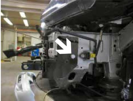
6. Hold base plate in place and align back holes with existing holes on frame, on both sides. Then insert 1/2-13 Whiz nut, with 10 inch wire, into opening on frame end to align with existing lower back hole of base plate, tighten 1/2-13 hex bolt and lock washer, on both sides. While maintaining a level position for the attachment tabs, tighten all bolts. **Be sure and use Loctite red on all bolts before tightening. Tighten all bolts according to torque chart in the General Instruction sheet.**
