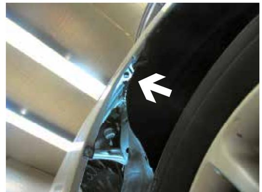
4. Just forward of front tires, on fascia's corner, remove one metric bolt with the 10MM socket, on both sides, pull fascia's corner to the side and forward, set aside.
