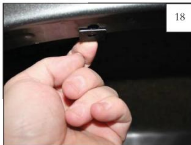
Install Clip (CL1-0022) over existing hole.
