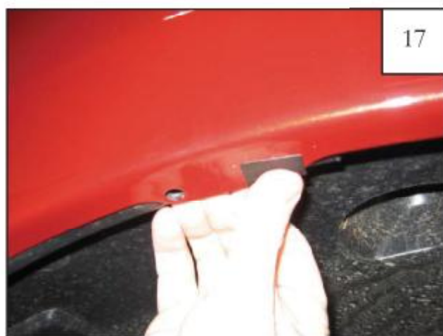
Install plastic tab over existing factory hole.
