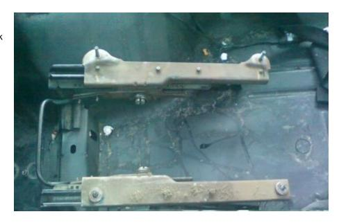
2. Once both seats are removed, place the PRP seat adaptors onto the factory studs with the angle pointing up. (note: the wider adaptor plate should be on the inside toward the tunnel) Insert the factory nuts loosely to allow adjustment of the seat.
