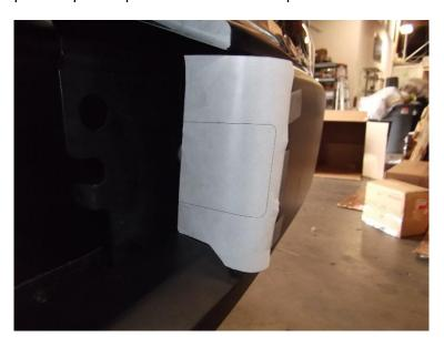
**Step 3:** Use a scribe or a punch and poke through the template to mark the pod at the center point of the corners.
