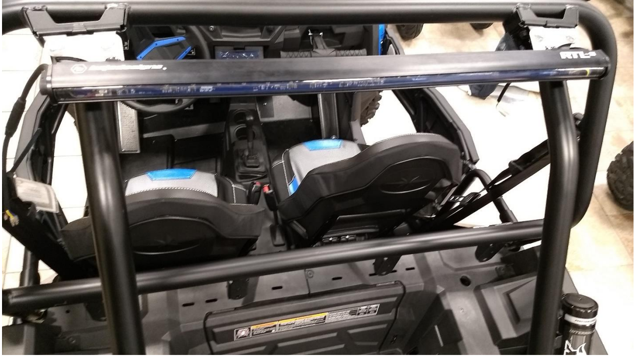
Mounting Bracket Orientation (tabs toward middle and bolts towards front of vehicle)
