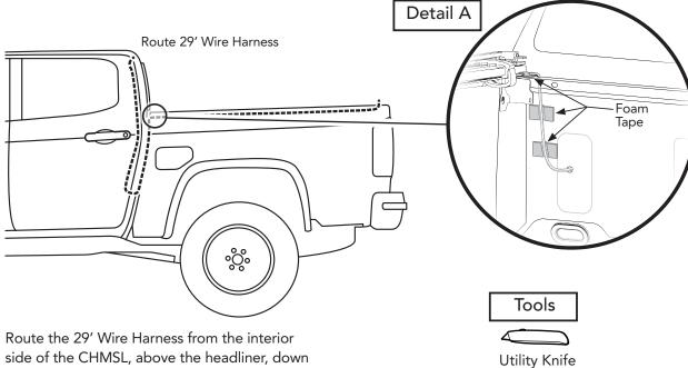
Route the 29' Wire Harness from the interior side of the CHMSL, above the headliner, down the rear driver side pillar, under the carpet, through the cab vent, into the vehicle bed, and along the top of the bed, underneath the bed rail cap. See Detail B.
