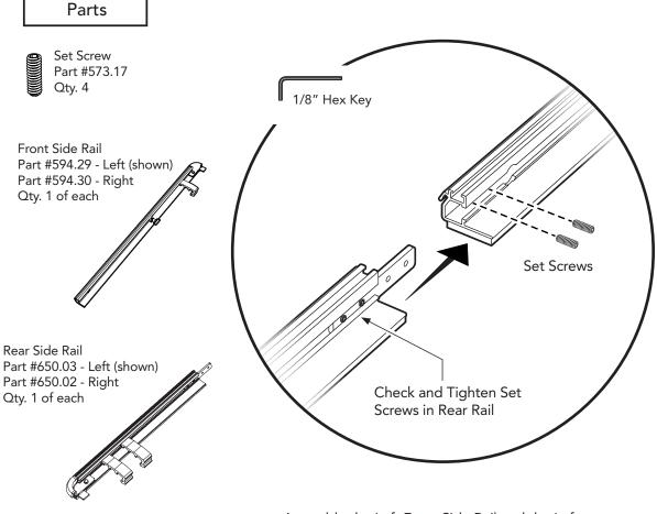
Assemble the Left Front Side Rail and the Left Rear Side Rail.
