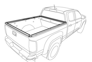
Attach Driver Side Bow Stack to Passenger Side Bow Stack.
