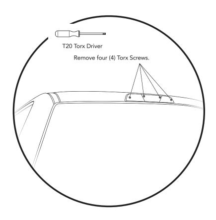
Use a T20 Torx Driver to remove the 4 screws that attach the Center High-Mounted Stop Light to the vehicle cab, and remove the CHMSL.
