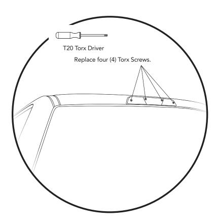
Find the four (4) T20 Torx screws you removed earlier, and re-attach the Center High-Mounted Stop Light (CHMSL) to the vehicle cab.
