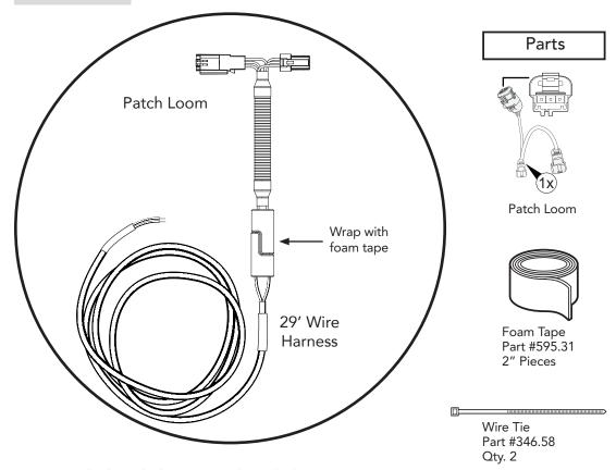
From outside the vehicle, connect the Vehicle Patch Loom to the 29' Wire Harness.
