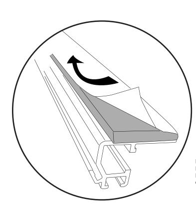
Locate the Foam Tape on the Left and Right Side Rails, and remove the paper backing from the foam tape.
