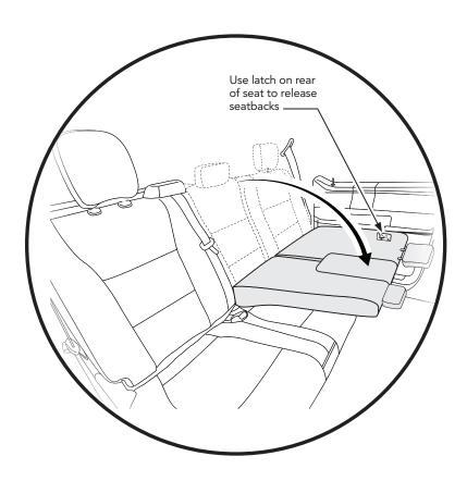
Use the latch on the rear of the driver side rear seatback to release the driver side and middle seatbacks, and flip both seatbacks forward.
