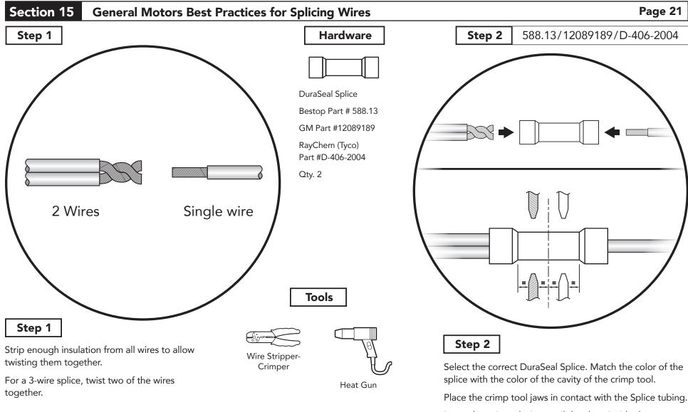
Insert the stripped wires until they butt inside the DuraSeal Splice. Crimp the wires in place on both sides of the DuraSeal Splice.
