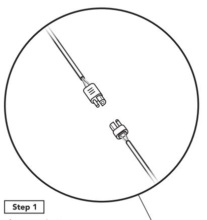
After routing the 29' Wire Harness using either Option 1 or Option 2, plug the 2-conductor connectors at the ends of the CHMSL Wire Harness and the 29' Wire Harness together.
