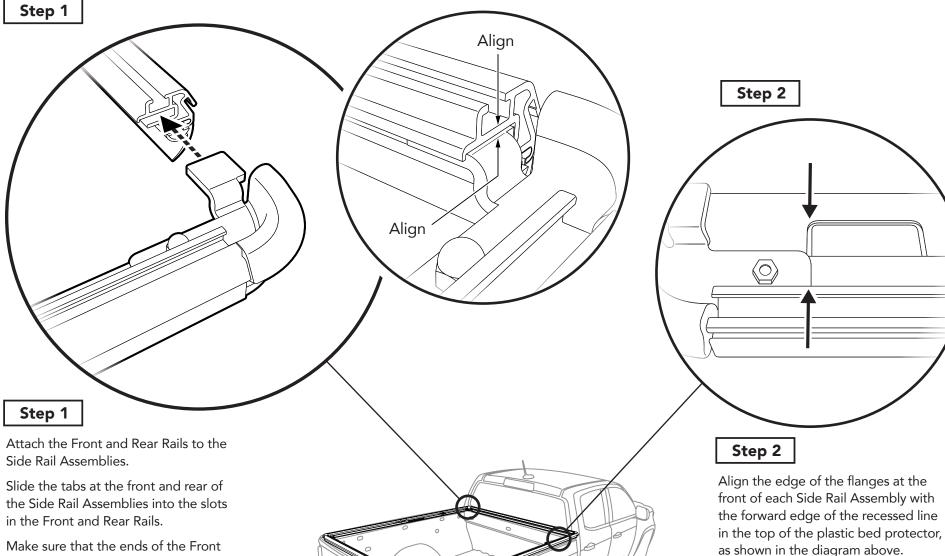
Make sure that the ends of the Front Rail and Rear Rail extrusions are aligned with the tongue of the attachment feature, where the tongue bends, and the small corner protrudes.
