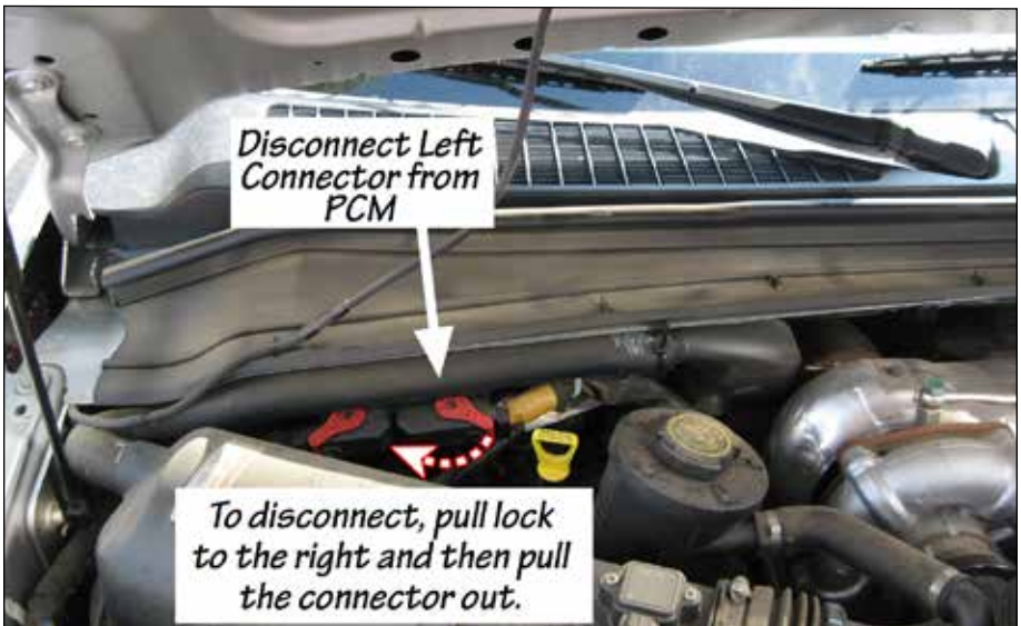
Figure 3: PCM Location on Passenger side.
