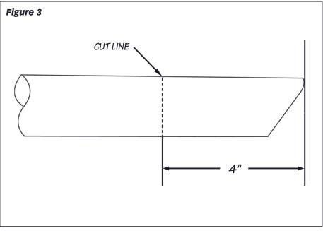
past the edge of the body or where aesthetically pleasing. Torque the band clamp to 35 ft-lb.
