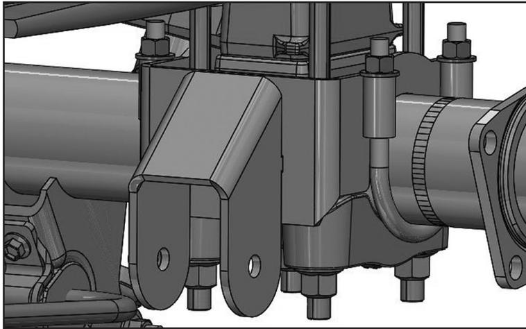
11. Repeat axle bracket installation on the passenger's side of the vehicle.
