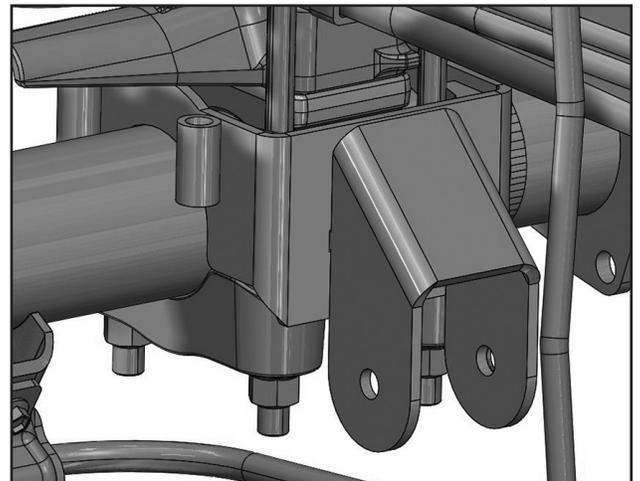
10. Locate two of the 1/2" U-bolt and install around the axle and up through the sleeves in the axle mount bracket (02886). Using the 1/2" fine thread nut and 1/2" SAE washer from Bolt Pack 962, tighten the U-bolts so that the axle mount clamps around the axle. The axle mount bracket should be parallel with the leaf spring perch. Tighten the 1/2" fine thread hardware to 45 ft-lbs.
