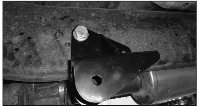
32. Slide the frame bracket as far back towards the axle as it can go in the slots in the frame. Mark the location of the three holes on the frame.
