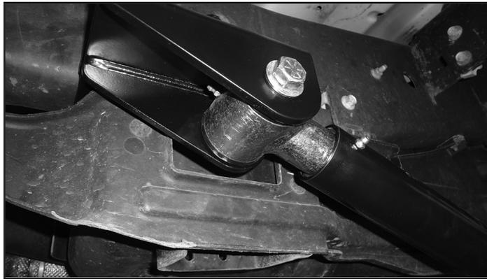
26. Repeat installation on the driver side using the passenger's side frame mount bracket (02878). Some models have a wire harness on the passenger side. First un-clip the wire harness from the frame near the slot to gain slack. See Figure 12.
