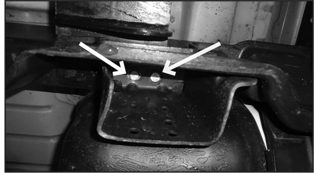
17. Install the driver's side frame mount bracket (02877) with the provided 3/4" x 1-1/2" bolt, 3/4" SAE washers, and 3/4" nut from Bolt Pack 961 through the hole on the bracket and into the slot on the frame. Leave hardware loose. **2011+ Models Only:** The bracket will be sandwiched in between the frame and fuel tank shield support as shown in Figure 9.
