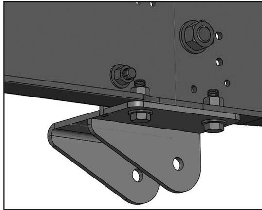
36. Models with a wire harness on the passenger side will use the provided mountable zip ties (tree on the end) to route the wire harness above the passenger side bracket. Mark two locations to drill a 7/32" hole to attach the mountable zip ties that will hold the wire harness above the bracket. See Figure 21 for a guideline as to where to drill the holes.
