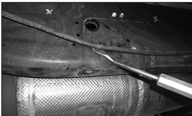
27. Install the 3/4" x 1-1/2" bolt, 3/4" SAE washers, and 3/4" nut through the hole on the bracket and into the slot in the frame.
