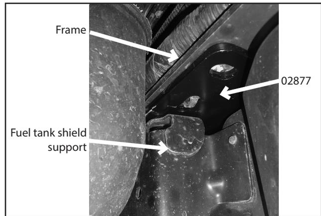
19. **2011+ Models Only:** Install the two provided 8mm x 45 mm bolts and 5/16" USS washers from Bolt Pack 961 through the two holes in the fuel tank shield support, sandwiching the frame mount bracket (02877) between the frame and fuel tank shield support. Leave hardware loose. *Note: Make sure the 8mm U-Nuts in the frame line up with the holes in the bracket and fuel tank shield support.*
