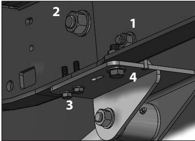
25. Attach the traction bar slider end (02869) to the frame bracket using a 9/16" x 4" bolt, 9/16" nut and 9/16" SAE washers from Bolt Pack 964. *Note: The traction bar slider end will slide out of the Recoil Traction Bar to attach to the frame mount. If it cannot slide out far enough, spin the bar so that it un-threads from the Forged Flex End.*
