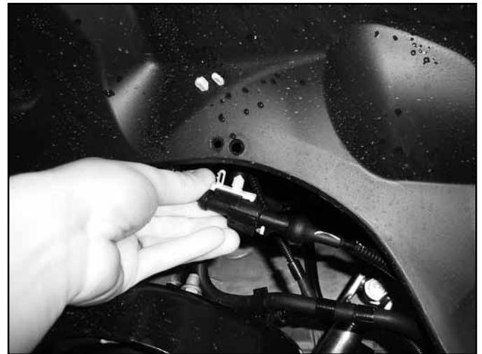
8. Disconnect the hub vacuum line from the hub (Fig 3).
