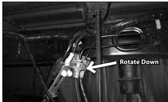
92. Attach the brake line to the relocation bracket with a 1/4" nut and 1/4" USS washer (BP #774). It may be necessary to rotate the OE brakeline clip bracket to have the lines face 'down' for adequate slack. Torque to 15 ft-lbs.
