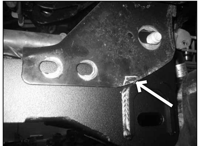
33. With the crossmember installed mark the differential hole on the factory control arm bracket. Remove the crossmember and drill a 5/8" hole at the mark, for easiest access drill the hole from front to back, a step drill is recommended for this step.
