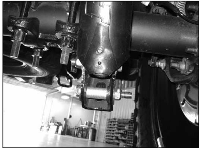
86. Install the new provided lift block so that the bump stop wing goes toward the inside of the vehicle. These blocks are side specific to slightly offset the axle forward. 02429 is the driver's side lift block, 02430 is the passenger's side.
