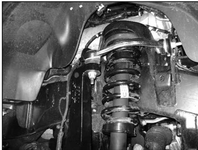
57. Torque the upper strut nuts to 35 ft-lbs. The lower bolt will be tightened later with the weight of the vehicle on the suspension.
