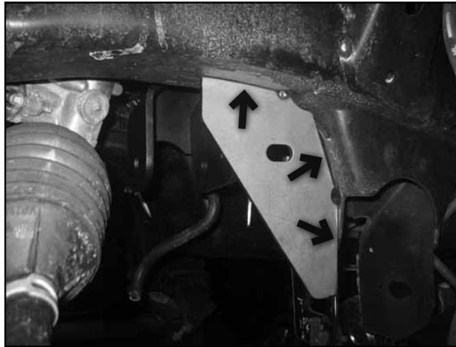
35. Temporarily install the differential drop bracket on the driver's side with OE bolt. Place the driver's side differential support bracket (L-shaped bracket) up between the weld in plate and differential drop. If the slots align, remove differential drop bracket and L-shaped bracket. Weld the outside of the plate in the 3 places shown. (Fig 17)
