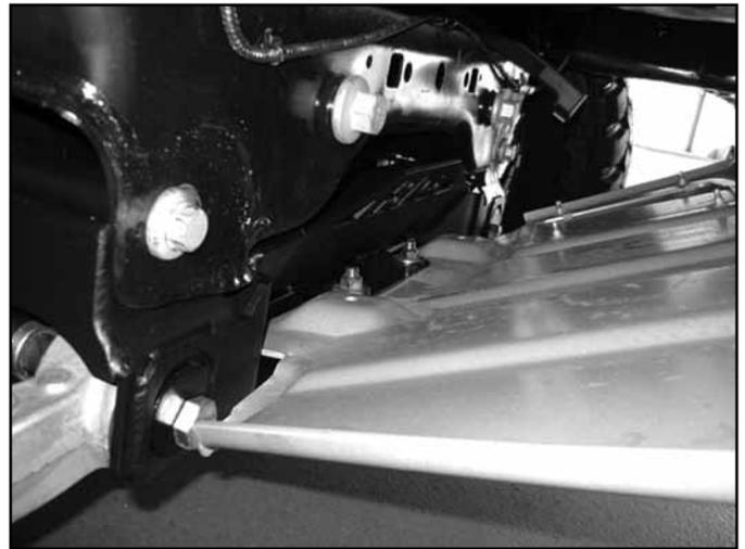
70. Reinstall front skid plate with 1/2" hardware and 10mm hardware with spacers. (#675) Tighten 10mm hardware to 35 ft-lbs, 1/2" hardware to 55 ft-lbs.
