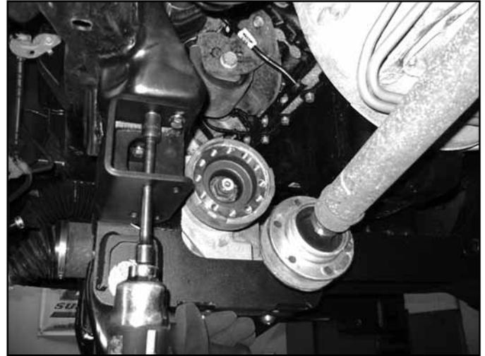
46. With the lower control arms installed torque the four crossmember mounting bolts to 222 ft-lbs. Ensure that the front crossmember is centered in the vehicle. Torque the differential skid plate bolts to 65 ft-lbs. Tighten sway bar drop hardware to 35 ft-lbs.
