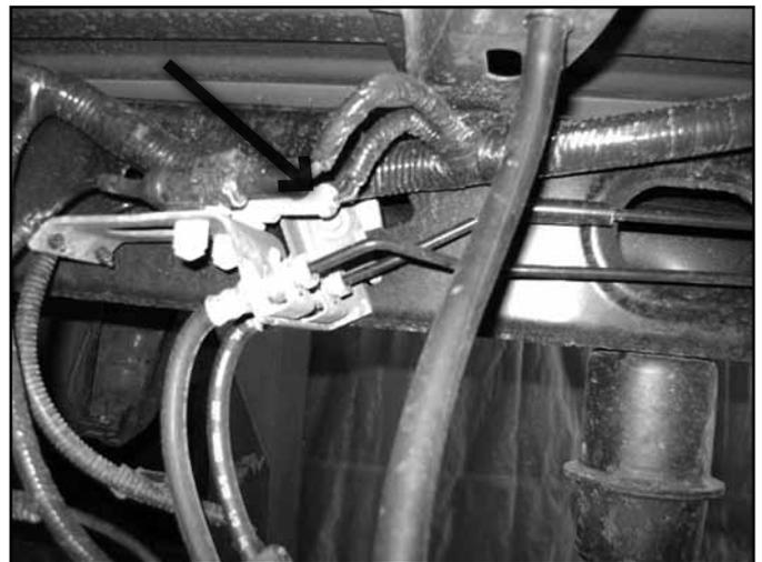
81. Support the rear axle with a hydraulic jack. Remove the OE shocks. Retain mounting hardware.
