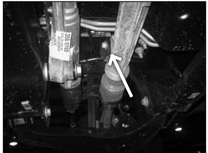
26. Pull down on the differential breather hose to gain additional slack.
