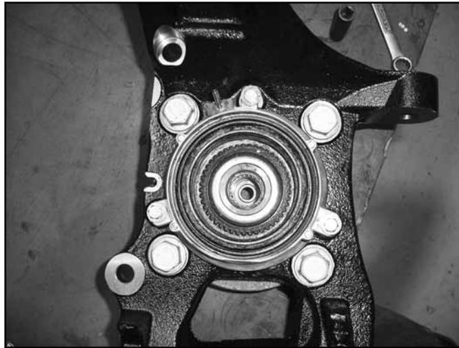
54. Install the dust shield with the factory 6mm bolts, tighten bolts securely (about 5-7 ft-lbs). Route the ABS cable behind the dust shield.
