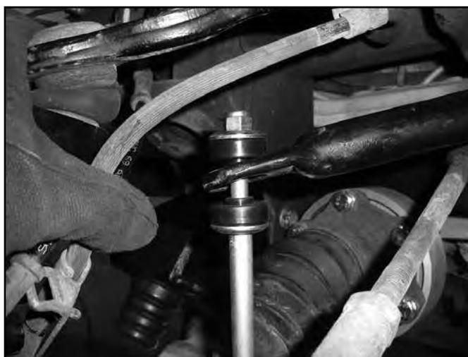
45. Attach the tie rod ends to the knuckles. Fasten with the original nuts and torque to 37 ft-lbs.
