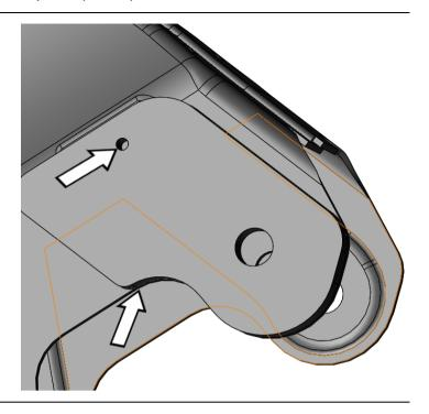
9. Drill pilot hole on the radius arm using 0.25" drill bit.
