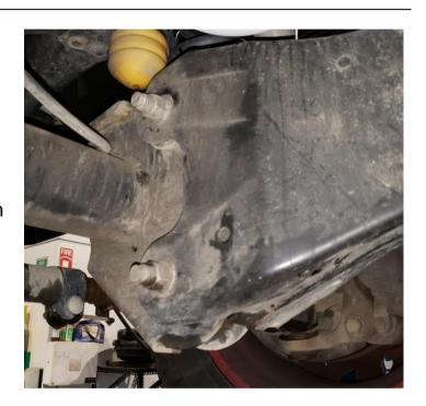
4. Removing the front two bolts on the radius arm, will release the arm from the vehicle.
