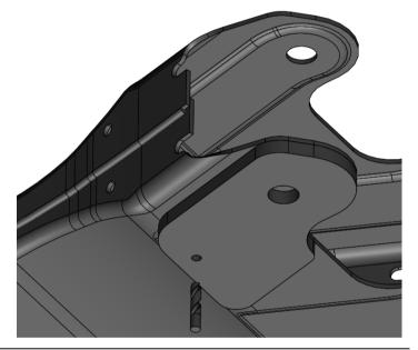
10. Put the supplied M6 bolt (FT-0161815) and M6 nut (FT-90700) through drilled hole and tighten.
