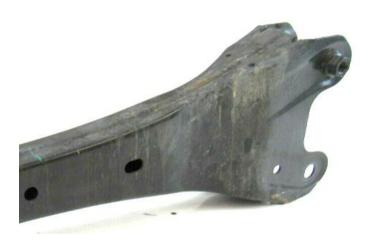
The adjustment slot must be 7. added to the top hole on the radius arm.
