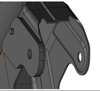
11. Drill the radius arm using supplied Ø3/4" hole saw.
