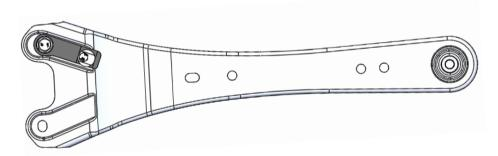
Remove the ABS wire support brackets from both radius arms.
