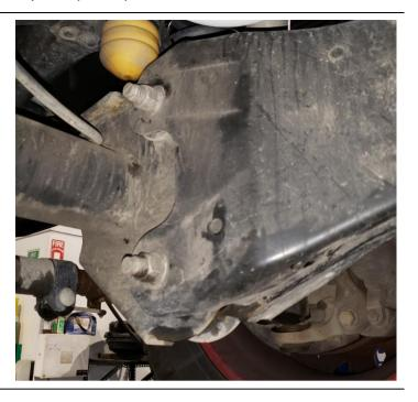
19. Using a 21mm wrench, rotate the eccentric washer in the keyway
