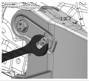
21. Once the desired castor has been reached, place the square washer (1302112-6) into the keyway on the castor adjuster plate (1302112-2).
