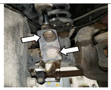
NOTE: Only loosen the bolts at this time. DO NOT REMOVE.
