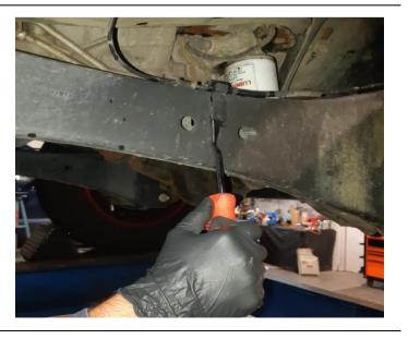
2. Remove the lower mounting bolts on the shock absorber from both sides of the vehicle. (18mm socket) then move the bottom of the shock out of the mount.
