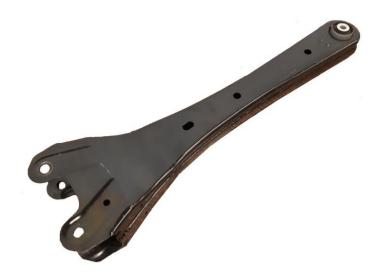
6. The driver's side radius arm will require the weld-nut to be ground flat. Cut the weldments off and arind flush.
