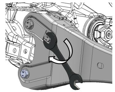
20. The orientation shown is the maximum caster angle that can be reached.
