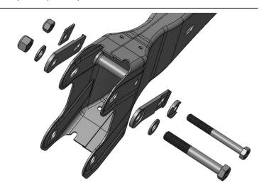
16. Place radius arm on the truck and install the M18 bolts. Use the supplied longer M18 bolt (FT-11114467), M18 nut (1302109), and M18 washer (1302110) through the new castor plates.
