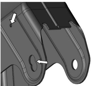
Re-mount the drill jig and repeat for the second side of the same radius arm.
