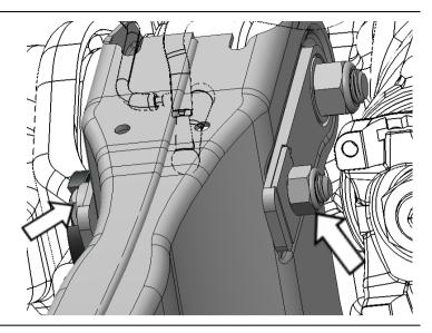
24. Tighten the upper, lower M18 radius arm bolts and nut.
