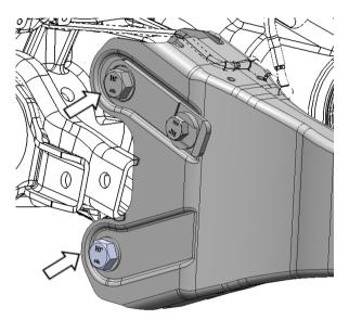
25. Tighten the rear radius arm bolt and nut.
