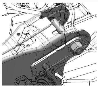
22. The square washer (1301221-6) has max angle mark to align with the mark on 1301222-2. This indicates the max angle.
