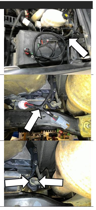
Connect the BD harness inline and carefully zip tie the harnesses so that they stay away from the exhaust pipe.
