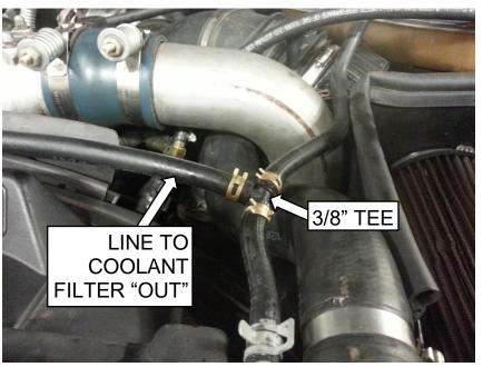
11. Route 3/8" hose from the tee fitting to the coolant filter head "OUT" securing with hose clamps. Be sure to secure with zip ties to avoid chafing.
