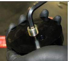
4. Before placing the filter head on the bracket. Assemble the straight NPT and ball valve and thread into the "IN" port, using sealant or pipe tape on threads.
