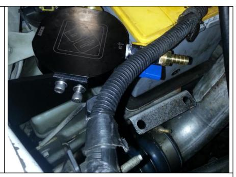
8. Cut a section from the heater hose running parallel to the intake runner and install the 3/4" x 3/8" x 3/4" tee fitting using the supplied gear/spring clamps.
