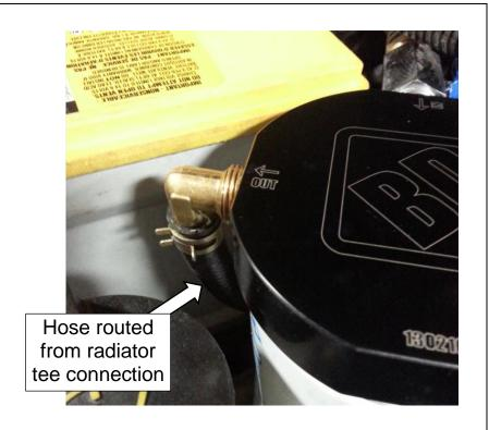
Ensure hoses routed properly and secured with zip ties and hose clamps.
