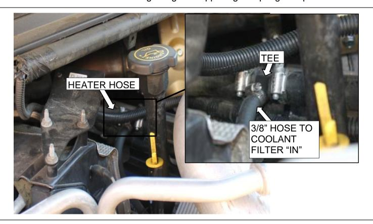
Route this hose to the port marked "IN" on the coolant filter head. Securing with hose clamps and zip-ties as necessary.
