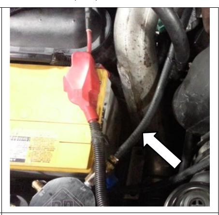
10. Cut coolant hose from degas bottle to radiator a few inches from radiator as shown. Install 3/8" tee fitting and secure with supplied hose clamps.
