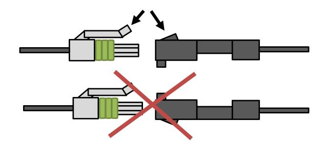
**2003-2004 Dodge 5.9L (CR)** – Locate the engine crankshaft position sensor, located toward the front of the engine on the left side beside the harmonic balancer. Cut off and discard the supplied three pin connector from the blue wire on the BD wiring harness (this is used only up to 2002). Tap the blue wire into the crankshaft sensor wire from pin 3 of the connector. Solder this connection and cover with heat shrink for longevity.
