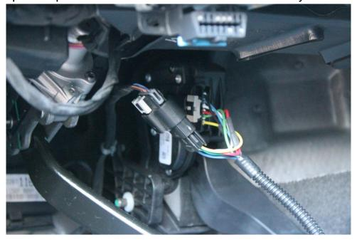
4. For 98.5-04 Dodge kits, disconnect the control knob harness from the main wiring harness. Route the two wire switch harness and white wire through the firewall and reconnect it to the main wiring harness. (Not required on other models).
