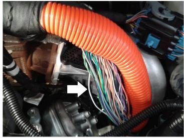
**2017-2022 GM L5P** – Locate the 8 pin sub-harness disconnect on the top of the engine for the crankshaft position sensor. Locate the solid green wire in pin 3. Remove some harness tape to have some wire to work with. Attach the light blue wire here for RPM pickup. Solder the wire and cover with heat shrink for longevity. Rewrap with tape when complete.
