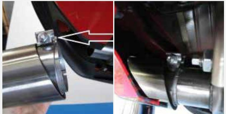
Slide the 3" band clamp onto the Vari-Tune exhaust tip with the bolt and nut facing towards the center of the vehicle and slide the Vari-Tune exhaust tip onto the outlet pipe of the BBK Vari-Tune muffler.
