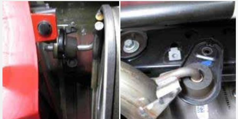
Remove the 2 bolts that secure the exhaust mount to the chassis located by the muffler tip. Next remove the bolt on the exhaust hanger that is located by the rear differential cross member. Once all 3 bolts are removed lift up on the exhaust and unhook the mounts from the chassis and remove the stock axle back from the vehicle.
