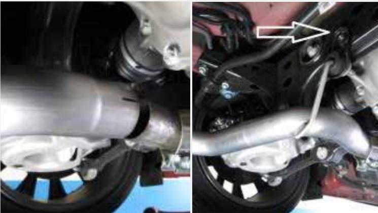
Slide the 2 1/2" band clamp and the BBK Axle Back tube over the stock exhaust pipe. Lift upward on the axle back tube and hook the exhaust hanger to the chassis.
