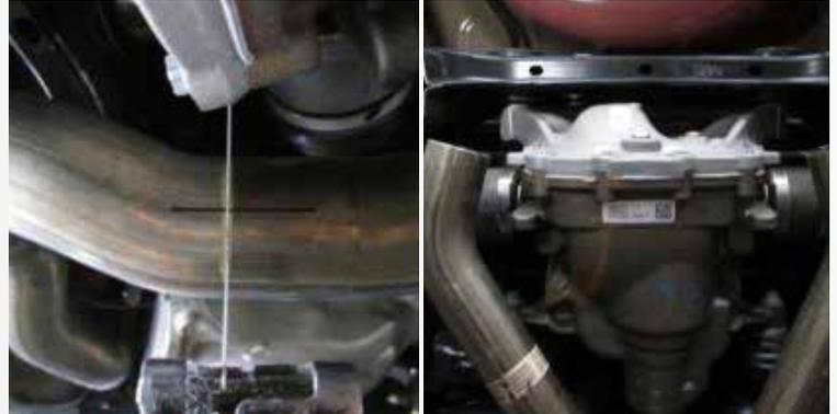
Using a saws-all cut the stock exhaust along the marked lines. When both passenger and driver side are cut your end result should look like the picture on the right.
