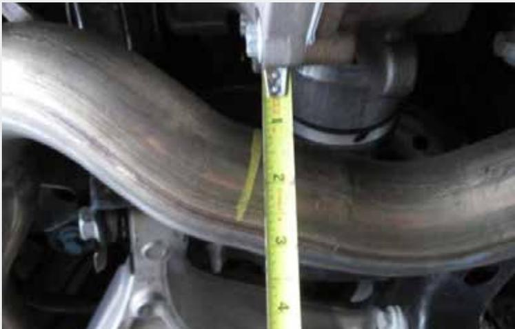
Mark the exhaust pipes in line with the rear differential cover plate. Make sure to mark a straight line with the angle of the exhaust pipe.
