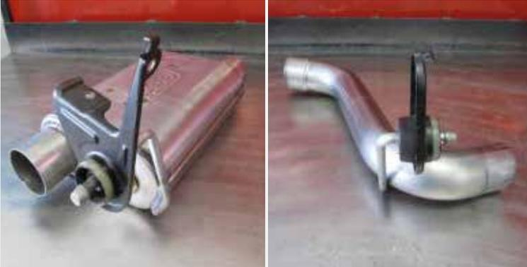
Working on the driver side, Remove the rubber exhaust mounts from the stock exhaust and install them accordingly to the BBK Axle Back System.
