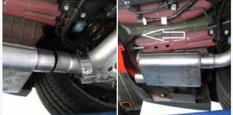
Slide the 3" band clamp and the BBK Vari-Tune Muffler onto the axle back tube. Lift upward on the muffler and hook the exhaust hanger to the chassis, reinstall the exhaust mount bolts and tighten them down.
