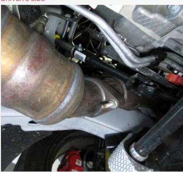
Disconnect O<sup>2</sup> sensor plugs and then remove factory head pipe using 16mm socket.
