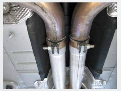
Using 15mm socket disconnect and remove factory head pipes.
