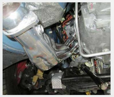
Install BBK headers using supplied hardware and gasket with 10mm socket/ wrench. Re-install motor mount and steering shaft.
