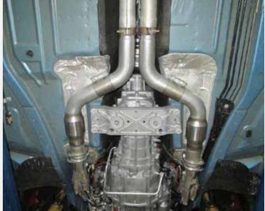
Now after headers are installed install supplied head pipe assembly the driver side and passenger side are labeled with little stickers on exhaust.
