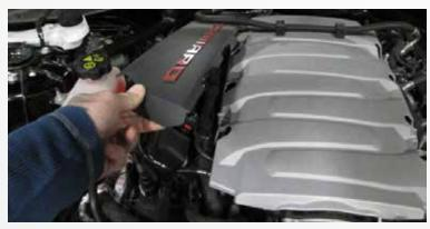
Remove the engine decorative covers from the engine by simply pulling them upwards released them from there mounting points.
