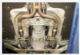
Install all (4) oxygen sensors and connect the wiring harnesses. Reconnect the negative battery terminal and enjoy the sound and power of the BBK full length headers "REMINDER" check coolant levels after
