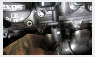
Disconnect all of the spark plug wires and spark plugs from the engine on the driver and passenger side of the engine.
