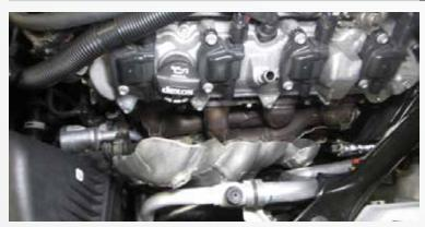
Remove the (3) bolts that hold the heat shields to the exhaust manifold on the driver and passenger side of the engine and remove the heat shields from the vehicle.
