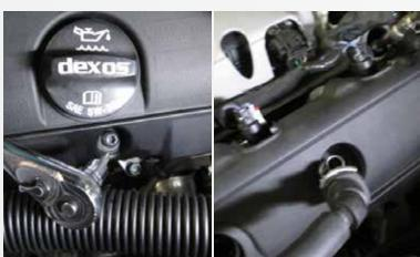
Remove the (2) Torx bit screws on the driver and passenger side coil covers. On the driver side remove the oil cap. Disconnect the vacuum tube that goes into the valve cover on the driver side and passenger side. Once the vacuum tubes are off lift up on the coil covers and remove them from the vehicle. Replace oil cap so no debris will enter the engine.
