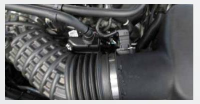
Disconnect the mass air flow sensor from the air inlet tube. Disconnect the vacuum tube located next to the mass air flow sensor. Using pliers disconnect the sound tube from the barb fitting located on the top of the air inlet tube. Loosen the clamp that holds the air inlet tube to the throttle body. Unclip the sound tube from the side of the air box. Disconnect the inlet tube from the throttle body and lift up on the air box to release if from its mounting points and remove it from the vehicle.
