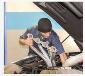
Driver-side installation. From underneath the vehicle lift the BBK full length header into place re-use the stock exhaust gasket. Start (2) bolts to hold the header in place that are supplied in the kit. From underneath the hood of the vehicle start the rest of the
