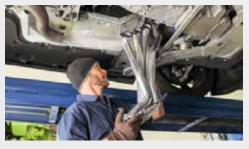
On the passenger-side of the engine. Remove the bolt that holds the dipstick to the cylinder head. Remove all exhaust manifold bolts.
