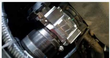
Reinstall the (4) bolts and tighten them down, install the wiring harness to the BBK throttle body and tighten down the hose clamp on the inlet tube to the throttle body, connect the negative battery terminal.
