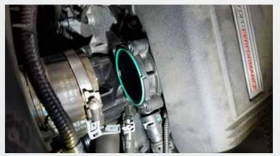
Remove the throttle body from the vehicle, wipe off any dirt or debris from the intake gasket before installing the BBK throttle body.
