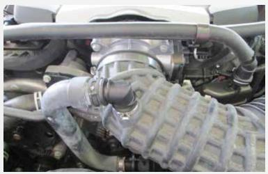
Remove factory air box tube using pliers, screw driver, 10 mm socket and wrench.
