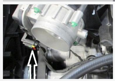
Disconnect the wiring plug from the throttle body, remove the (4) bolts that secure the throttle body to the intake manifold.
