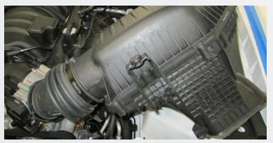
Remove air box from the vehicle. NOTE: on charger models only remove the crews that hold the air box lid to the lower half and remove the lid and inlet tube from the vehicle.
