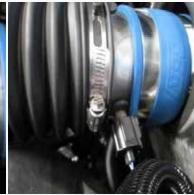
Install the rubber o-ring into the adapter pipe, remove the Air Temp sensor from the stock air box and install it into the adapter tube. Install the BBK adapter tube into the inlet tube. Install the BBK coupler and supplied clamps onto the BBK air filter, install the BBK Air Filter through the hole in the air shield. Next slide the air filter onto the adapter tube once you have it in position tighten down all of the clamps.
