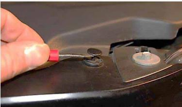
Remove the plastic radiator cover by prying up the center of the plastic pin heads at the slots cut on each side pull all the pins out and set the cover to the side.
