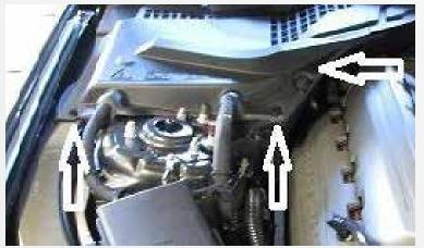
Remove the 3 screw pins that hold the battery cover to the body lift up the battery cover and disconnect the negative battery terminal. Remove the engine cover by pulling it upward releasing it from its rubber grommets.
