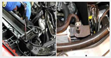
Remove the 2 10mm bolts from the driver side radiator mount and remove the mount by pulling it upwards from the vehicle. Install the BBK Air Filter Shield into place by setting it straight down onto the radiator mount peg. Install the stock bolt through the air shield and bolt it back into the small tab on the inner fender. Reinstall the upper radiator mount and tighten the 2 bolts.
