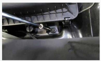
Remove the 10mm bolt on the right side of the air box that mounts it to the inner fender. Detach the air box from the lower inlet tube on the side of the radiator as you remove the air box. By pulling upwards and towards the firewall.
