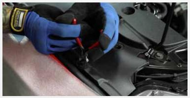
Remove the plastic radiator cover by prying up the center of the plastic pin heads at the slots cut on each side pull all the pins out and set the cover to the side.
