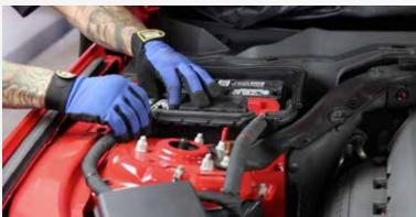
Re-install the engine cover and the radiator cover. Reconnect the negative battery terminal.
