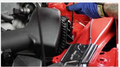
Remove the 10mm bolt on the right side of the air box that mounts it to the inner fender. Detach the air box from the lower inlet tube on the side of the radiator as you remove the air box. By pulling upwards and towards the firewall.
