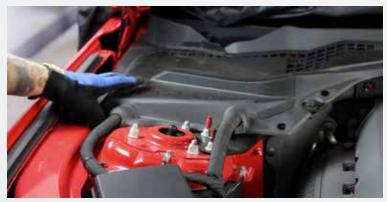
Place the battery cover bock onto the battery and reinstall the 3 screw pins.
