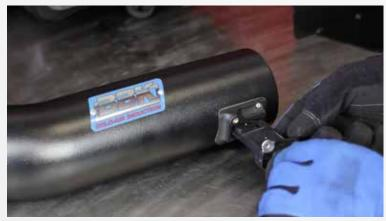
Remove the Mass air sensor from the stock air box and install it into the BBK Cold Air Tube using the supplied hardware. (The sensor will only go in one way) Install the angled BBK coupler with the vacuum port in it onto the throttle body. Install the supplied vacuum adapter onto the hose and insert it into the hole on the side of the BBK coupler.
