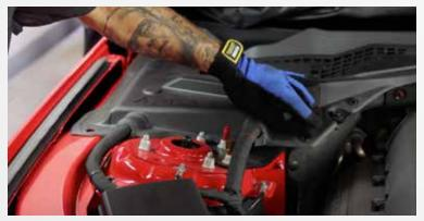
Remove the 3 screw pins that hold the battery cover to the body lift up the battery cover and disconnect the negative battery terminal. Remove the engine cover by pulling it upward releasing it from its rubber grommets.
