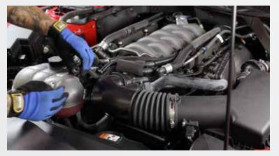
Disconnect the 3 breather hoses and the sound hose from the inlet tube. Loosen the clamps on the inlet tube at the throttle body and the air box, remove the inlet tube from the vehicle.
