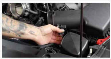
Unplug the Mass Air Sensor. Detach the Mass Air Sensor wire harness from the side of the air box by slightly pulling on the harness on the barbed mounting pin.
