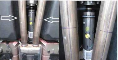
Use a straight edge and mark the bottom side of the pipes be sure to make the cut marks in line with the pipes they should look like the pictures above not straight across from each other because then you will be cutting the pipes at an angle.
