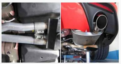
Level out the BBK Resonator Delete and the stock mufflers using approved jack stands or preferably muffler stands.
