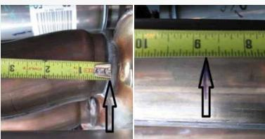
On the passenger side measure from the edge of the weld straight back and make a mark at 8 34".
