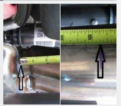
On the driver side of the resonator measure from the edge of the weld straight back and make a mark at 9 <sup>1</sup>/<sub>4</sub>".
