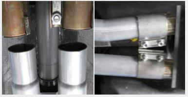
Lift the BBK Resonator Delete into place and slide the front portion into the stock barrel clamps.
