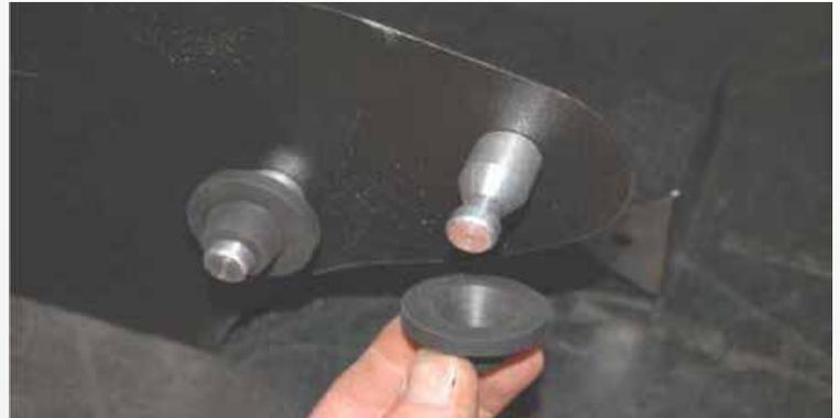
Assemble the 2 aluminum pins to the bottom of the BBK air filter shield using the supplied ¼-20x ½" Phillips screws. Install the stock rubber grommets onto the pins.
