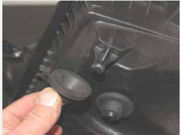
Remove the bolt on the right side of the stock air box that mounts it to the inner fender. Detach the air box from the lower inlet tube on the side of the radiator as you lift the box out to remove. Detach the Mass Air Sensor wire harness from the side of the air box by slightly pulling on the harness at each barbed mounting pin. Remove the 2 rubber grommets from the bottom of the air box.
