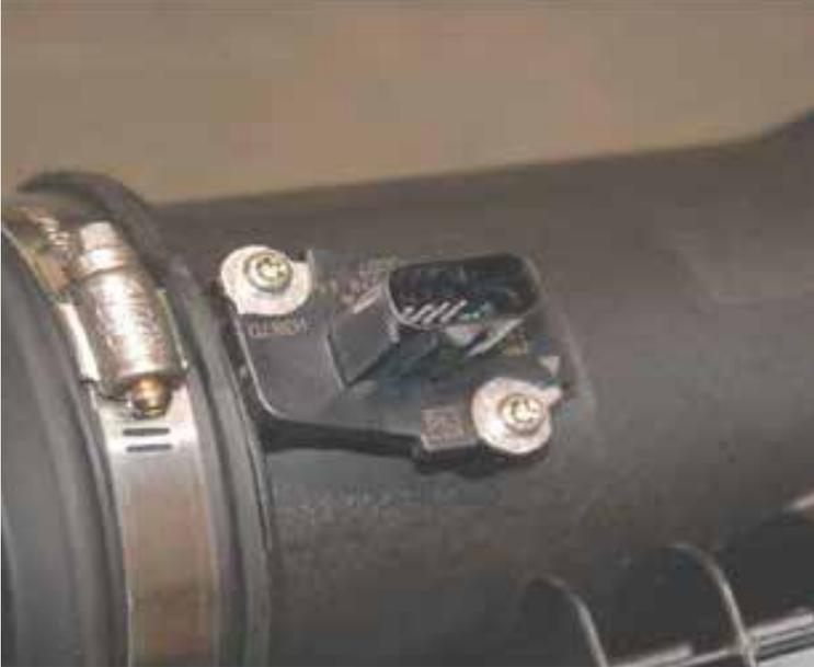
Remove the Mass Air Sensor from the stock air box tube. Install in the aluminum mounting base on the BBK inlet tube with the 2 supplied 4mm
