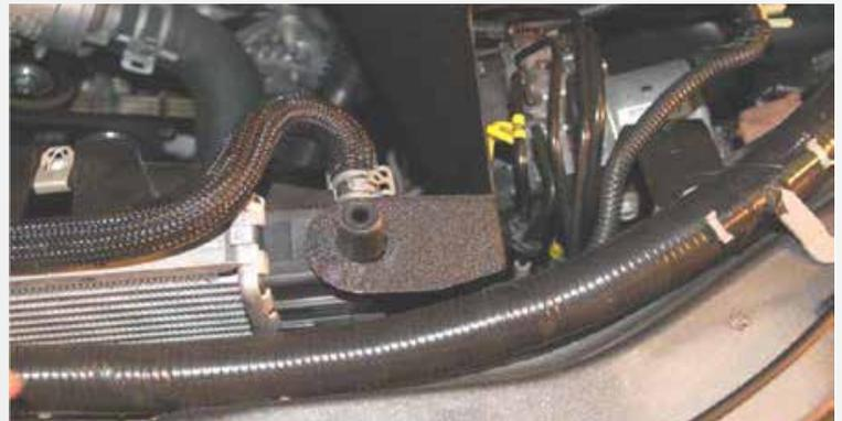
Install the BBK air filter shield into place and position over the radiator mount peg with the rubber grommets seating into their holes in the inner fender. Install the stock bolt back into the small tab on the shield and tighten the bolt. Re-install the upper radiator mount and tighten the bolts.
