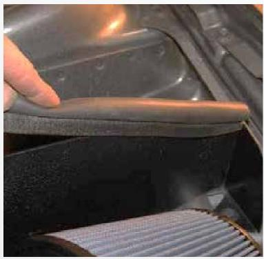
Install the supplied spongy trim to the top of the Air Filter Shield and cut off any excess trim.
