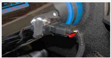
Remove the MAF sensor from the stock air box and install it into the BBK Cold Air Tube using the supplied hardware. (The sensor will only go on one way)
