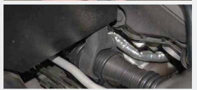
Route the sound tube under the plastic breather hose, so sound tube will pass under BBK cold air shield. Use the stock rubber clamp to retain the sound tube to the bottom of the filter shield.
