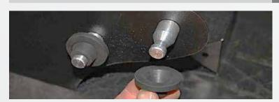
Assemble the 2 aluminum pins to the bottom of the BBK Air Filter Shield using the supplied 1/4-20x1/2" Phillips screws. Install the stock rubber grommets onto the pins.
