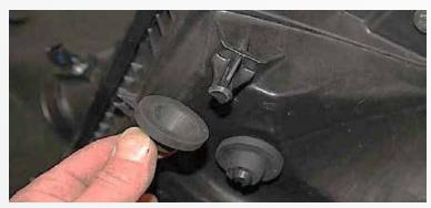
Remove the bolt on the right side of the air box that mounts it to the inner fender. Detach the air box from the lower inlet tube on the side of the radiator as you remove the air box. Detach the Mass Air Meter wire harness from the side of the air box by slightly pulling on the harness on each barbed mounting pin. Also remove the 2 bottom rubber grommet for the air box.
