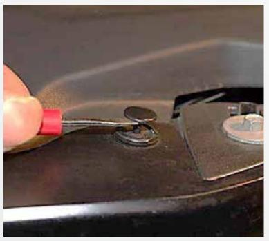
Disconnect the negative battery terminal. Remove the plastic radiator cover by prying up the center of the plastic pin heads at the slots cut on each side. Pull pins out and set the cover aside.
