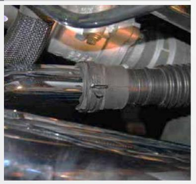
Install the 2 blue couplers to the BBK inlet tube. Install the tube thru the hole in the air filter shield then onto the throttle body. Connect the sound tube to the BBK inlet tube as well.
