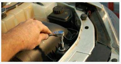
Remove the bolt that mounts the front of the air box to the vehicle. Lift out the air box and remove with the inlet hose.
