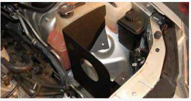
Place the filter shield into place in the engine compartment and line up the grommet with its hole. Mount the front tab of the filter shield using the stock bolt.
