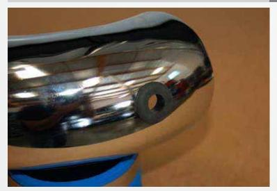
From the hardware kit, install the supplied rubber grommet into the hole in the BBK Inlet Tube. Install the Air Temperature Sensor into the grommet.
