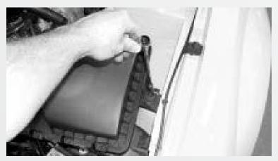
Loosen the hose clamp that attaches the inlet hose to the throttle body. Remove the bolt that holds the air filter box to the driver side fender-well.
