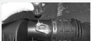
Remove the 2 torx screws from the mass air meter and slide the meter out of the stock inlet hose, and then install it into the BBK inlet pipe using the supplied screws.
