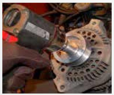
Remove the alternator mounting bolts, lift the alternator out of its cradle to access the pulley. Using an impact, remove the stock pulley and install the BBK Pulley. Re-use the stock nut and/or washer.
