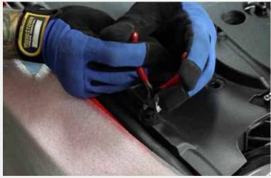
Remove the plastic radiator cover by prying up the center of the plastic pin heads at the slots cut on each side pull all the pins out and set the cover to the side.
