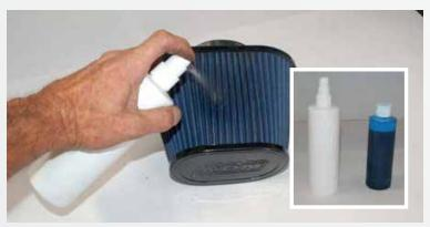
Wipe large debris from filter. Using the taller white bottle of cleaner from the kit, liberally spray the cleaner until it completely saturates the pleated mate-
