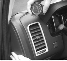
Be sure to secure the ecometer cable under your dashboard by utilizing wire ties, tape or other means. You do not want the wire to get in the way of your feet or pedal action. Run the ecometer cable up the side of your dashboard and push the cable into the trim to hide and secure.
