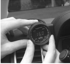
The ecometer dial face will rotate 350° degrees so you can achieve proper dial alignment and viewing angle. To rotate the dial, hold the back of the ecometer with one hand while you carefully rotate the bezel of the dial with your other hand. The ecometer will stay in whatever position you have rotated or indexed the dial to.
