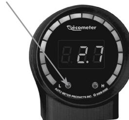
The ecometer's brightness level can be easily changed by simply holding down the left (mode) button. The ecometer will cycle through four brightness levels.
