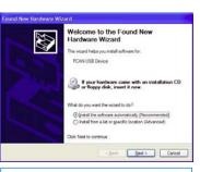
2. Windows will then display the New Hardware wizard. Make sure the Install the software automatically option is selected, then click the Next button to continue the hardware installation.
