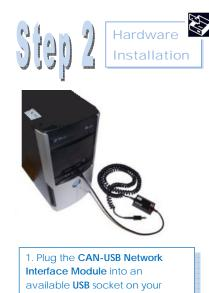
1. Plug the CAN-USB Network Interface Module into an available USB socket on your computer. Windows will detect that a new device has been connected and will display a message at the System Tray to report this.
