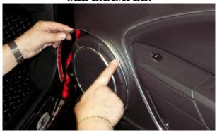
**5.** With the front surface tabs properly prepared simply remove the red release liner from the back of the new stainless grille overlay and carefully line up the six overlay tabs with the grille surround tabs and firmly press the new cover into position. Remove the protective liner.
