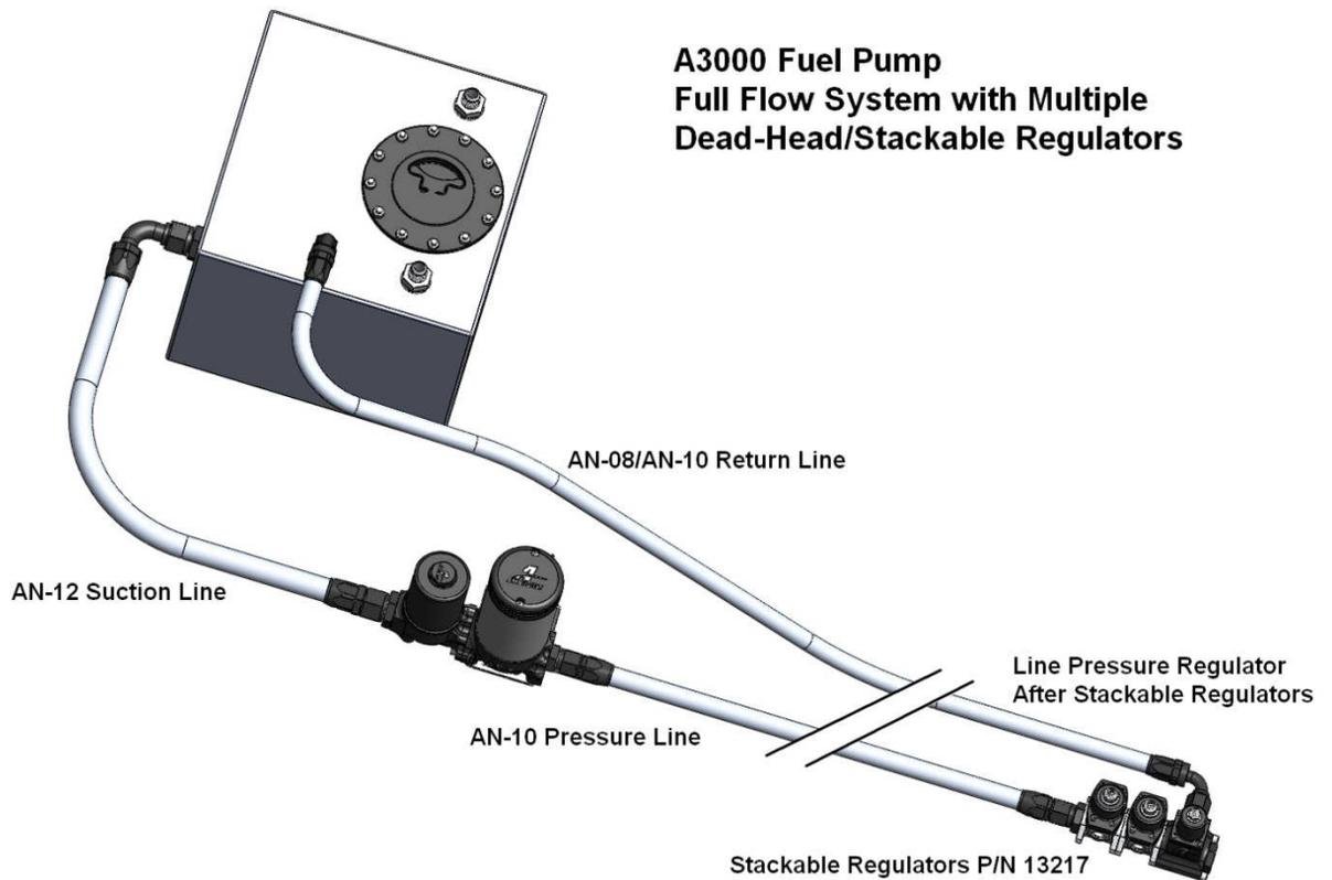
10. The HP Bypass Regulator may be coupled directly to the last Stackable Regulator using the included o-ring and fasteners. Thread the o-ring side of an ORB-08/AN-08 port fitting into the regulator return port and block the opposite (outlet) end with an ORB-10 port plug such as Aeromotive P/N 15617.
