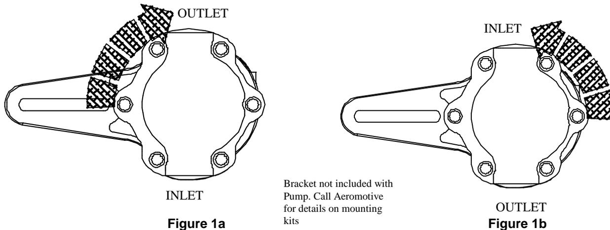
6. Connect the fuel cell sump to the fuel filter inlet, we recommend using fuel filter Aeromotive p/n 12304 or 12302, utilizing a minimum of AN-10 steel braided fuel line. Next, connect the fuel filter outlet to the fuel pump inlet utilizing a minimum of AN-10 steel braided fuel line, refer to Figure 1 for determining the fuel pump inlet.
