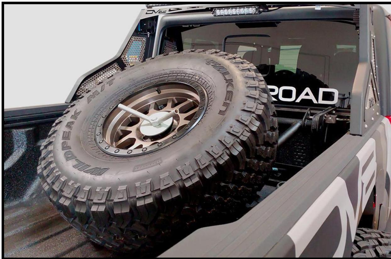
***NOTE: For 0+ offset wheels or 13.50"+ tires, you may need to flip over the tire and wheel to allow for proper fitment.***
