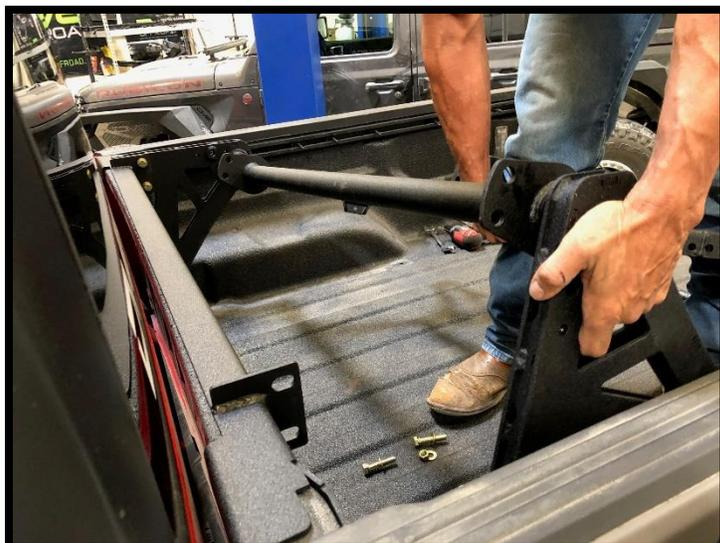
7. Tighten all hardware at this point. Main carrier tube should easily move up and down. Next, secure bolt pull locks into place using provided hardware. Make sure to put pull lock into one of two holes on main center tube before securing. **NOTE:** These may need to be tapped into place initially. This is normal.
