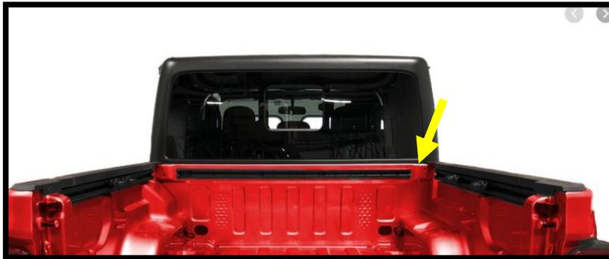
3. Attached the header board loosely with the supplied hardware as shown in the image.
