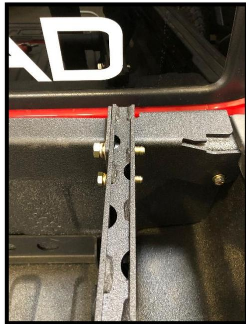
6. Install the main carrier onto the passenger side mount by slipping the main tube over the passenger mount tube. Then place the driver side mount into the main carrier tube and place it on the bed mounts and secure into place.
