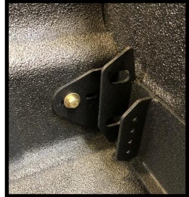
5. Once both support bars are installed, place the passenger side mount into place as show and loosely install hardware. This needs to be able to move to get the main carrier and driver side mount installed.
