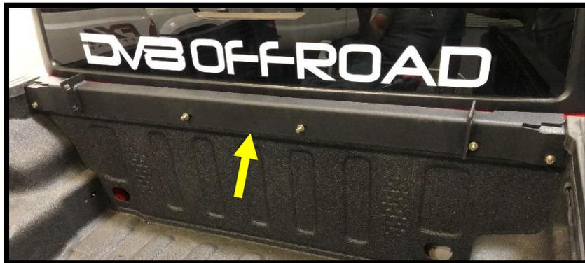
4. Install the lower support. The lower support has two holes on each side. The front hole with the factory threaded hole in the bed is required, the second hole that is through bolted is optional for tires larger than 40”.
