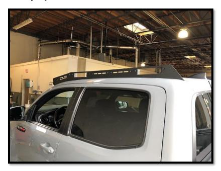
4. Peel back the tape and place each side of the rack over holes. (NOTE: When installing the bolts into the factory nutserts, place a small amount of silicone on the bolt to prevent leaking).
