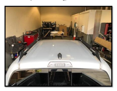
5. Beginning from the front (1) and rear (6) first, install the cross bars using supplied hardware. Be sure to leave all bars loose until they are all installed. (NOTE: You do not need to use the supplied spacers unless you are unable to install the rack without gaps in the cross bars).
