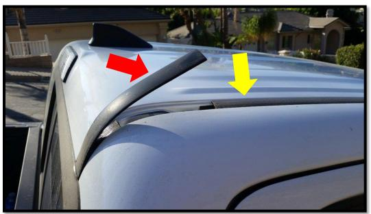
2. Them remove the main strip by starting from the back (yellow arrow) until fully removed.
