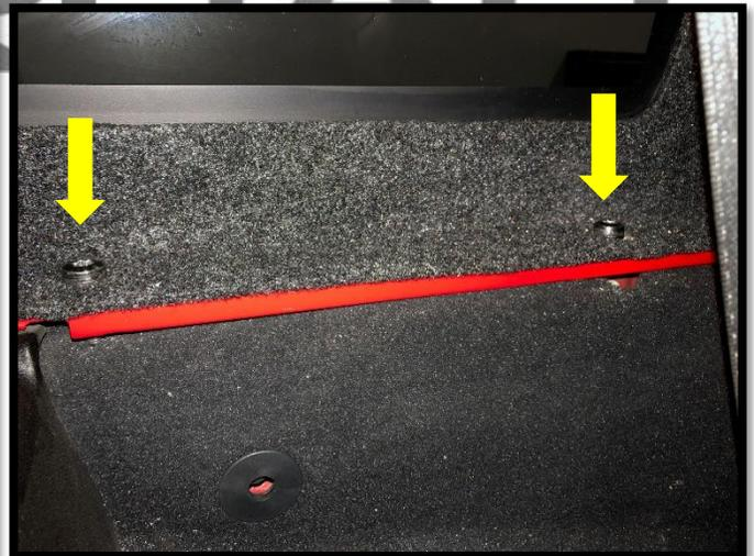
3. Install the rear section upper bolt shown below and tighten. These two bolts are located where the Targa installs over the B pillar. (4 Door Only)
