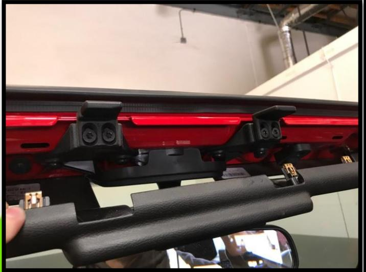
The front brackets will look like the photo below and will be marked with the letter L and R. The L bracket goes towards the driver's side and the R bracket goes to the passenger side. There will be threaded holes where these will install. The hardware that was sent will contain 4 bolts to connect these front 2 brackets. There may be paint in the holes that makes the installation of the bolts more difficult.
