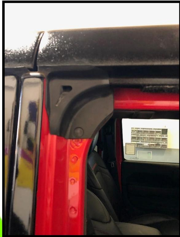
6. Be sure to push the front seals into position and make sure that they are not tucked under the top. (Images above)
