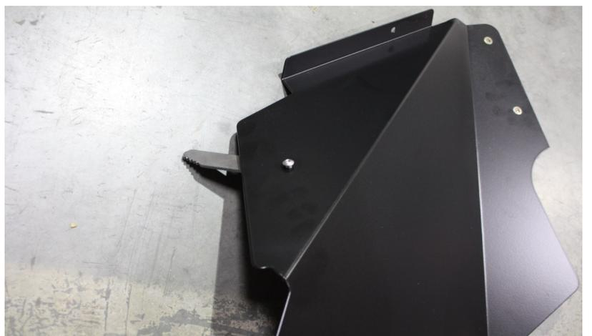
5) Place the liners in the fender location. You will use the factory hardware to attach to the Jeep at the four locations indicated by arrows. Cut and use the supplied adhesive rubber strip ( E ) to dampen any noise made from metal on metal contact if needed.
