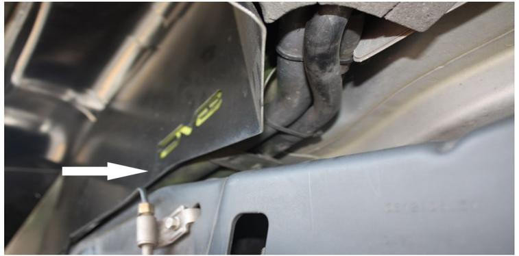
10) re-insert new liner and feed screws through. Use the wrench to hold nut in place.
