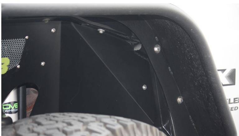
7) REARS : If necessary, jack up the Jeep from a safe place other than the axle to give yourself more room. Release the fender / liner combo by removing the push-in rivets from inside fender well and pulling upward on the fender to disconnect from snap-in clips.
