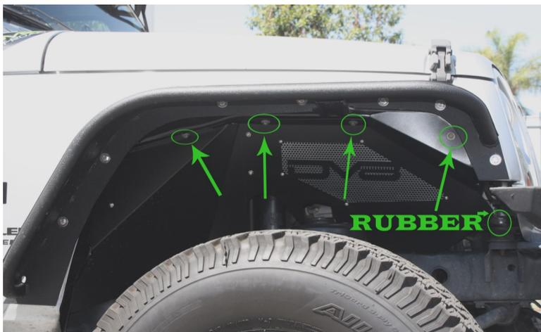
6) Once the inner fenders are aligned in the proper position, install with the factory hardware to secure inner fender. Tighten the screw near the fire wall while helping the arm to make contact with fire wall.
