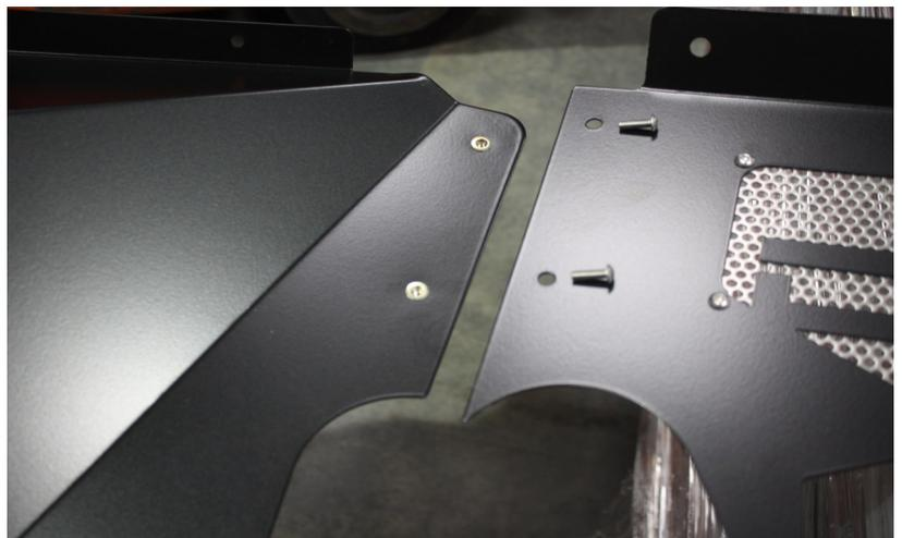
4) Attach the supplied arm (A) on the back of the hole closest to the firewall of the Jeep. Let it hang loosely. This arm will catch and secure on firewall.
