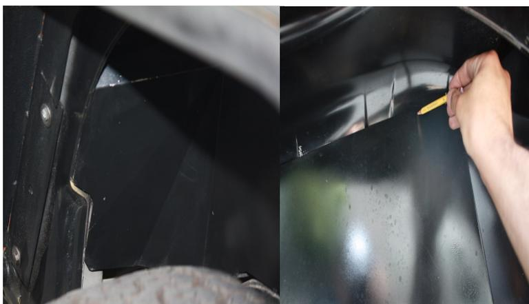
9) Proceed drilling locations (7/32nds) for the supplied screws and lock nuts ( D ) \*DRIVERS SIDE USE CAUTION HAVE SOMEONE HELP KEEP FUEL RELATED HOSES CLEAR FROM PUNCTURE.
