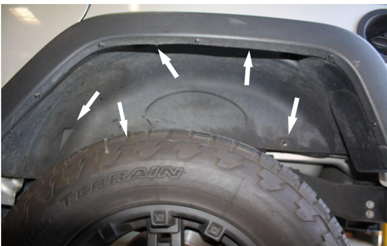
8) Install the new DV8 inner fender by flexing the liner and manipulating it in the opening. From there, a little force is needed to snap in place. Mark the 5 locations to drill with punch or marker. Than remove liner and proceed to next step.
