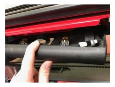
The ends of this panel are held in by bolts, after pulling the center portion down it is not necessary to loosen these bolts to access the bracket locations but if you want to then you can.
