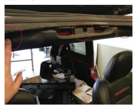
Install the 2 brackets using the supplied bolts into the OEM threaded holes.
