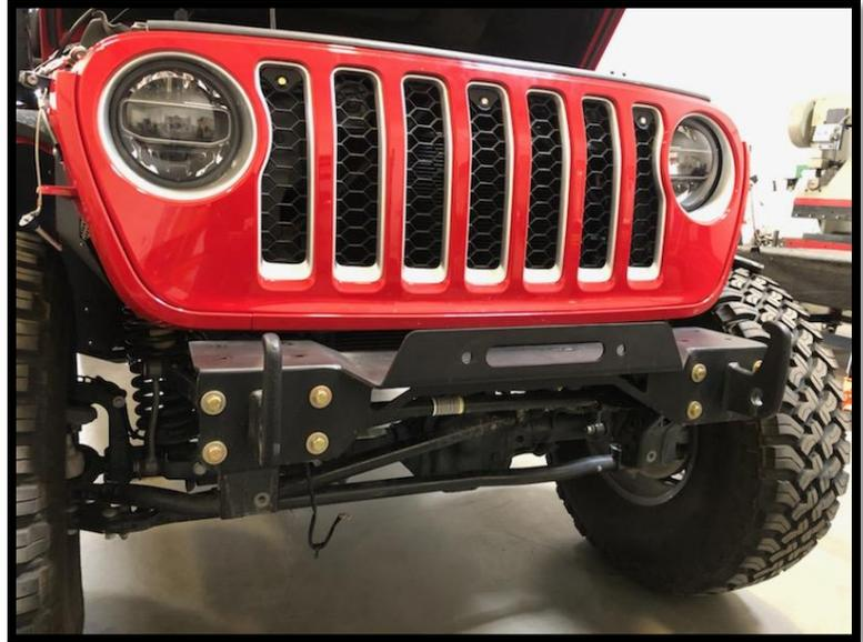
3. Once winch plate is secure, install the main center section of the bumper by sliding it over the top of the winch plate. The bumper should wrap over the D-Ring mounts like shown in image below.
