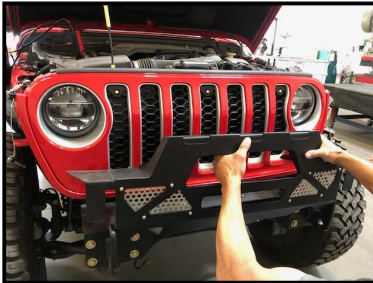
4. Align the 8 holes on the top of the bumper with the winch plate below. Secure the 4 holes closest to the center with our taper allen head bolts and rock washers provided in the hardware kit.
