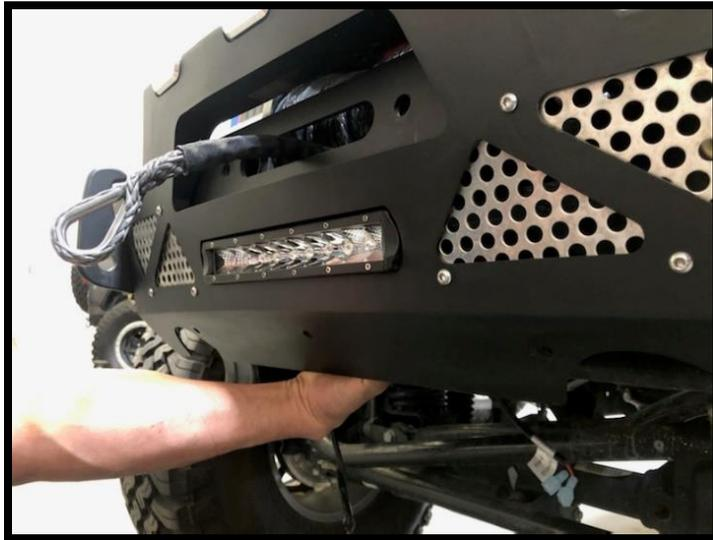
7. Install the wings (included stubby) or (full-width FBJL-02W) with the provided rock washers and hardware. The hole in the front of the stubby wing will remain open at this point.
