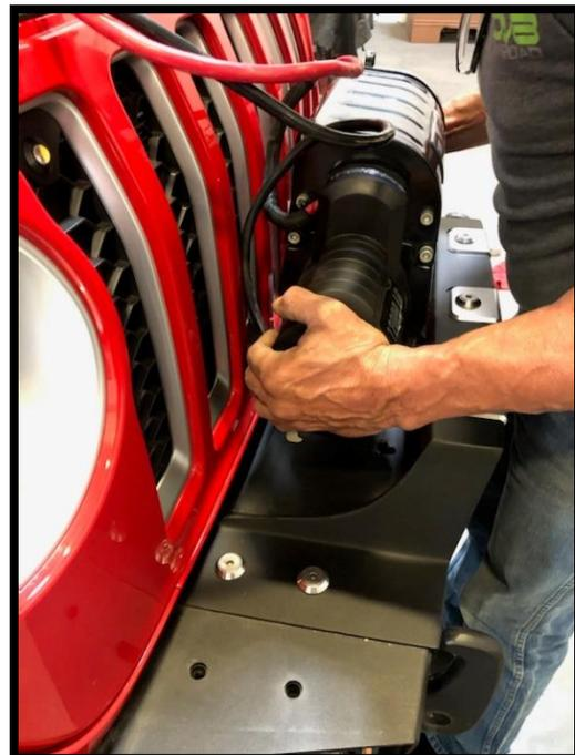
6. If you are going to install our BS6E30W5W, install the light now with the hardware supplied with the light.
