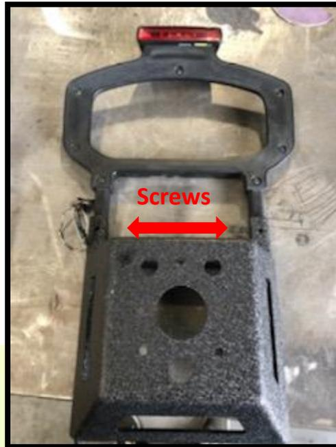
9. If you are running a rear camera you will utilize the factory camera bracket (plastic) and the provided camera enclosure. If you do not have a camera, you will utilize the block off plate.
