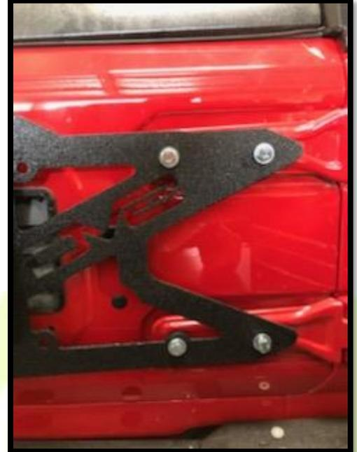
6. Once all (4) four bolts are in place, use factory hardware and remaining (8) eight spacer for bolts around tailgate exhauster vents.
