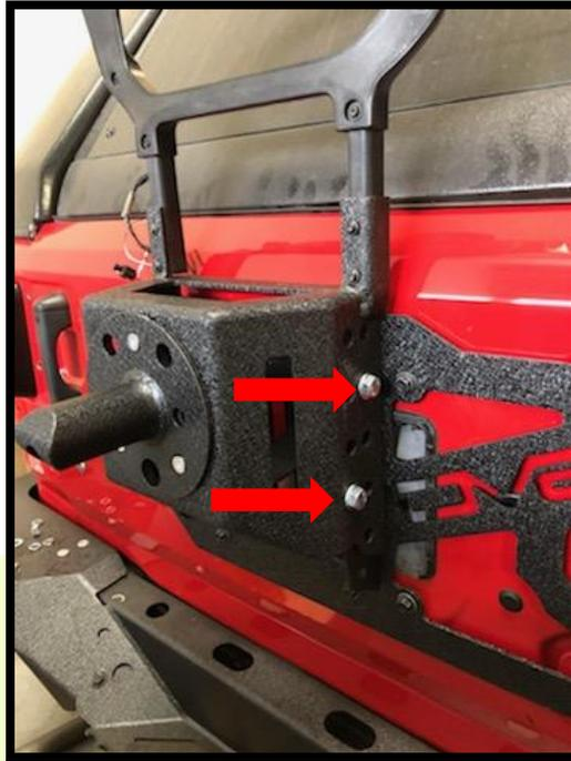
13. On each side of the carrier, place one bolt at the highest point on one row of holes, and one at the lowest point of connection with the tailgate plate and tire mount on the other row.
