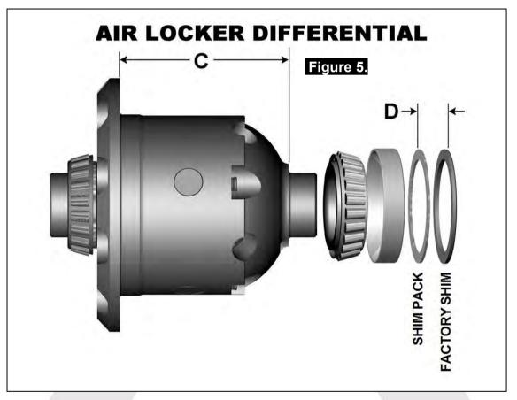
Measure the distance from the Air Locker bearing shoulder to the ring gear mounting face (shown as 'C' in Fig. 5.) and record this measurement as 'C'.
