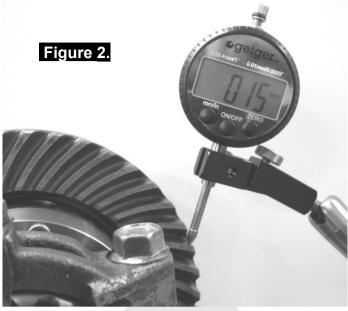
☐ While supporting the pinion gear by holding the drive flange, rotate the differential in both directions while observing the maximum variation in depth from the indicator (i.e., the highest value minus the lowest value). This value is referred to as the ring and pinion backlash.
