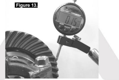
☐ Refer to your vehicle service manual for the specified maximum and minimum amounts of backlash. If the backlash is not within the specifications then the differential will have to be removed and reshimmed.
