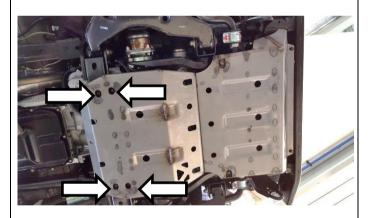
3. Loosely fit diff panel to chassis using 4x M8x1.25x25 bolts, spring washers and flat washers.
