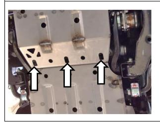
4. Loosely fasten 3x M8x1.25x25 bolts, spring washers and flat washers to join front panel to diff panel.
