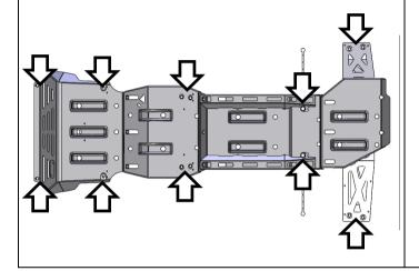
10. Tighten all fasteners joining panels to chassis.
