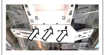
Loosely fasten transfer case panel to transmission panel using 3x M8x1.25x25 bolts, spring washers, flat washers and flange nuts.
