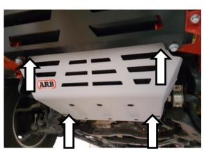
2. Loosely fit front panel to chassis using 4x M8x1.25x25 bolts, spring washers and flat washers.
