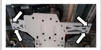
7. Loosely fit transfer case panel to chassis using 4x M8x1.25x25 bolts, spring washers and flat washers as shown.
