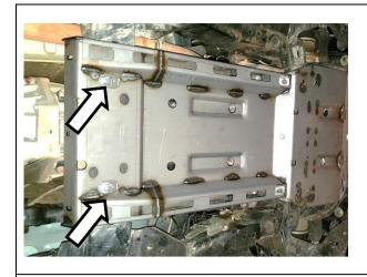
5. Loosely fit transmission panel to chassis using 2x M12x1.75x30 bolts, 2x M12 spring washers, 2x flat washers and 2x M12n nut plates.
