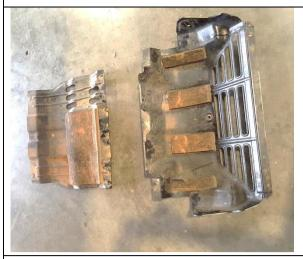
Remove OEM panels (front splash panel & diff panel) from vehicle – 6 bolts.
