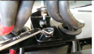
25. Using M8 fasteners fit control box mounting bracket to pan
