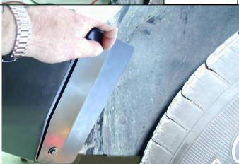
72. Fit liner retainer bracket with black M6 bolt and washer sets into M6 cage nuts in wing returns each side as shown.
