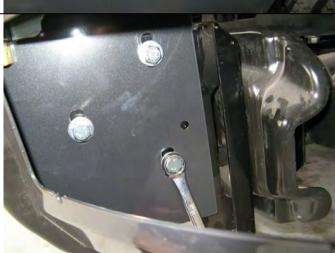
65. When bar is aligned, tighten bolts.
