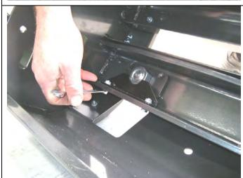
21. When the large nut is in its final position, secure with the nut retaining bracket using an M6 bolt, washer and flange nut.
