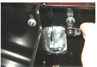
47. Slide the buffers down over the frame and secure using M6 flange nuts on the four lower buffer studs on each buffer and M6 nyloc nuts with large M6 flat washers on the two studs located on top face.
