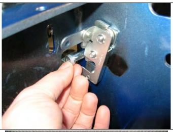
50. Fit the striker pin to the **RHS** hinge plate and secure with 5/16"UNC nut and spring washer as shown and tighten to 22Nm or 16lbft
