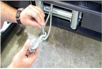
69. If winch fitted, fit off winch hook.
