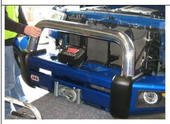
63. Using two people, three if winch fitted, position the bar assembly on the vehicle mounts.
