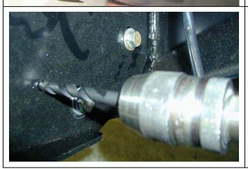
Osing the M10 pilot holes in mount brackets, drill pinning hole through uprights on bull bar. Fit M10 screw, washer set and flange nut and do up tight.
