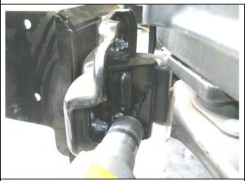
Drill 1 x M10 pinning hole in chassis using existing hole in reinforcing bracket as a guide.
