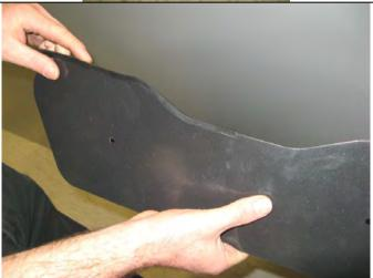
35. Wrap rubber extrusion around winch cover as shown starting from the centre of the back edge, trim off excess.
