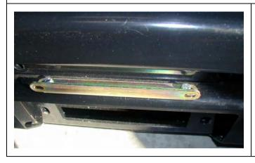
22. Secure the number plate bracket using M6 bolts, flat washers and flange nuts. Attach the longer side to the bullbar and the shorter side to the number plate.
