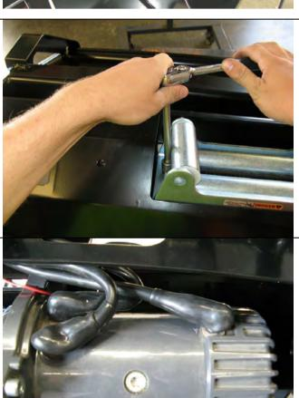
31. Fit the roller fair lead, pull only the end of the cable through and adjust the position of winch then bolt up securely. Use the 1 ½" long bolts in the top and 1 ¾"in the lower set through the RFL.
