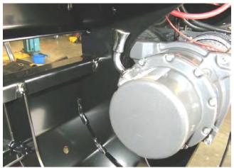
30. Position the winch with the mount face facing upward on an adjustable table or similar and with the assistance of another person lower the bulbar over the winch. The winch handle should be in the LHS of the bull bar for smaller winches than 12-15000lb winches which are on the opposite side as they spool in the opposite direction. The cable must always spool off the bottom of the winch.
