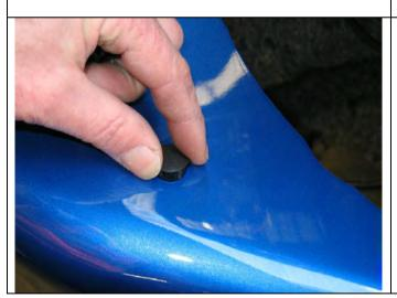
76. Unless fitting CB aerials, fit blanking plugs in provided holes in the top of the wings.
